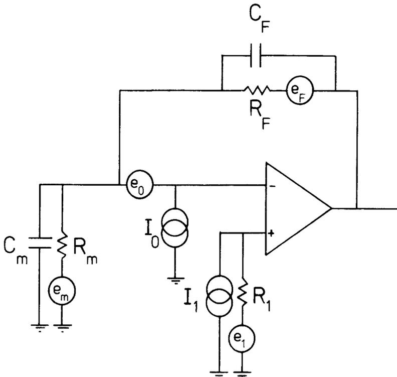
Fig. 1. Circuit diagram of the electronic setup.  $e_0$ ,  $I_0$  and  $I_1$  represent the voltage and current noise sources which take into account the noise behavior of the amplifier.  $e_m$ ,  $e_1$  and  $e_F$  are the voltage noise sources associated with  $R_m$ ,  $R_1$  and  $R_F$ , respectively
