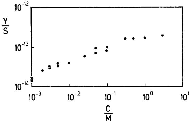
Fig. 6. Variation of  $\gamma$  as a function of the bulk concentration of KCl. Lipid: PC 16:4  $\text{CH}_3$ /cholesterol 1.0%/0.1%/n-decane. (w/v). Applied voltage  $V_m=97$  mV.  $T=25^\circ\text{C}$
