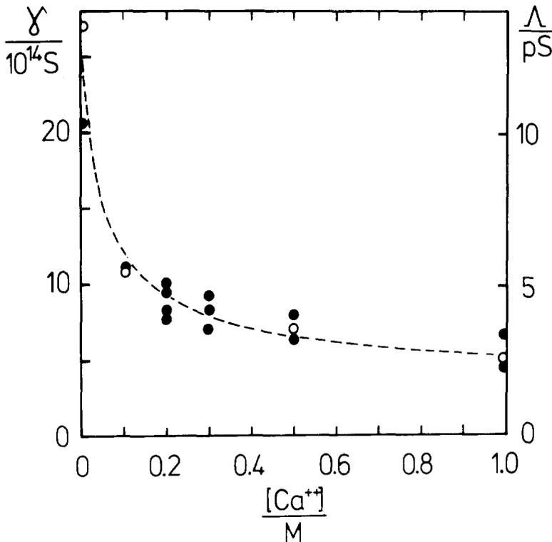
Fig. 7. Variation of  $\gamma$  as a function of the bulk concentration of  $\text{CaCl}_2$ . Lipid: PC 16:4  $\text{CH}_3$ /cholesterol 10%/0.1%/n-decane. (w/v). Electrolyte: 1 M KCl+various amounts of  $\text{CaCl}_2$ .  $V_m = 97.2$  mV.  $T = 25^\circ\text{C}$ . Filled dots: results obtained from noise analysis. Open dots: results obtained from single channel experiments
