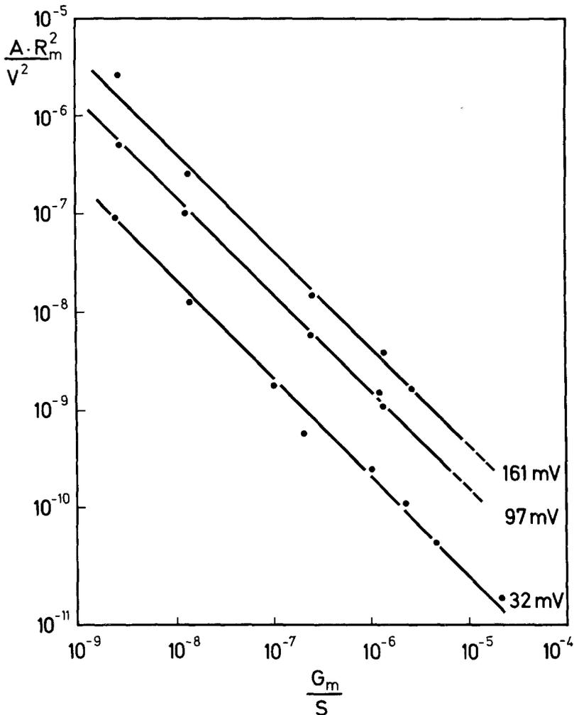
Fig. 5. Amplitude  $A$  of the  $1/f$  component of  $S_I(f)$  as a function of membrane conductance  $G_m = 1/R_m$  and applied voltage  $V_m$ . Lipid: PC 16:4  $\text{CH}_3$ /cholesterol 1.0%/0.1%/n-decane (w/v); electrolyte: 1 M KCl;  $T = 25^\circ\text{C}$
